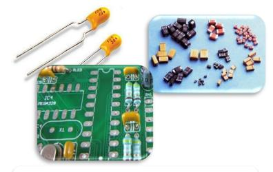
Ta capacitors – color/identification based labelling & easy to break connections
